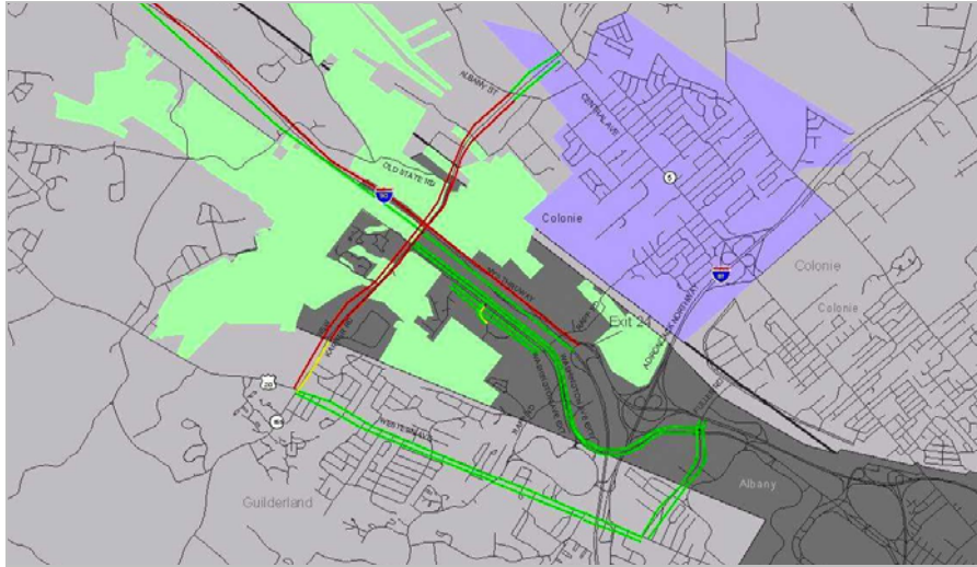
2000 PM Peak Hour Midblock Level of Service in the City of Albany and the Towns of Guilderland and Colonie, New York.
